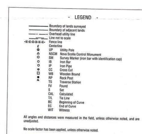
THE BEARINGS ARE: \_\_\_\_ MAGNETIC for the year \_\_\_\_ GRID based on the 3° modified transverse mercator projection having central meridian 64°-30' west and are referenced to Nova Scotia Control Monument numbers
